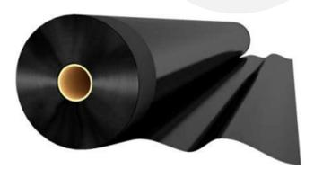
For best results, joints can be hot air welded with a twin wedge welder and tested with an air lance. Alternatively, double sided tape can be used for jointing.
